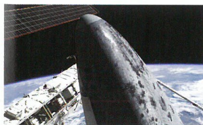
The tiles on the nose cone of the space shuttle contained graphite
